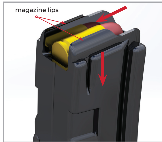
Figure 16: Loading the magazine
