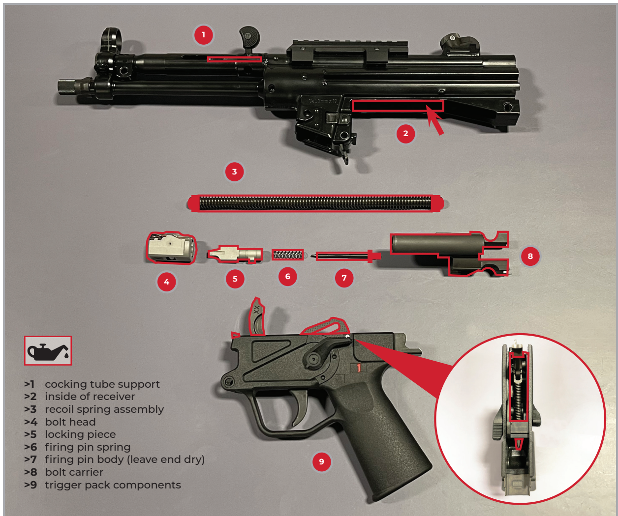
Figure 37: ZF-5 lubrication points
