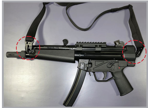
Figure 7: Mounting the carrying sling to the ZF-5
