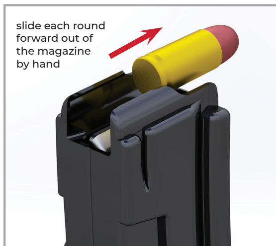
Figure 22: Unloading the magazine
